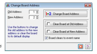
You may not know the address programmed into a board and it may not show it because it is displaying the last data sent to it. Fortunately, any board will respond to a command sent to address 0 (zero) regardless of the board's programmed address. Thus you can enter zero for the old address and the desired address in the new address field. Clicking the Change Board Address button will program the new address into all connected boards.
